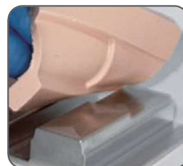
No material fracture Maximum peel strength → 0.5N / 25 mm
