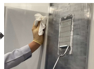
Laminate peel ply on glass cloth
